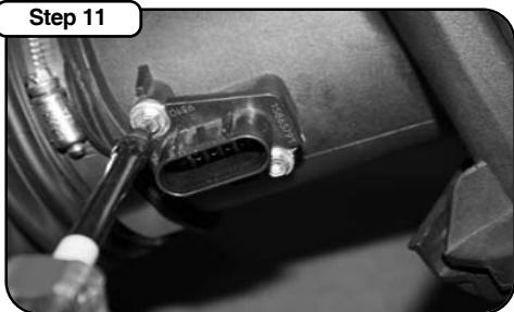
Remove MAF sensor from stock air intake tube.
