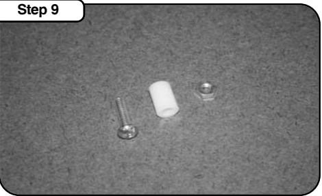
View of lower housing mount parts (screw, nylon spacer, nut).
