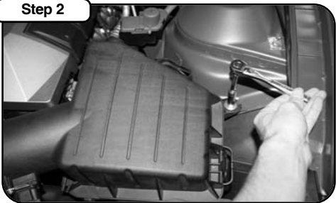
Remove nut from right side of air filter housing.
