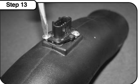
Install MAF sensor in aFe air intake tube using supplied 8/32 screws.
