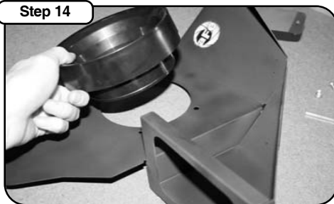
Install air filter adapter on aFe housing.
