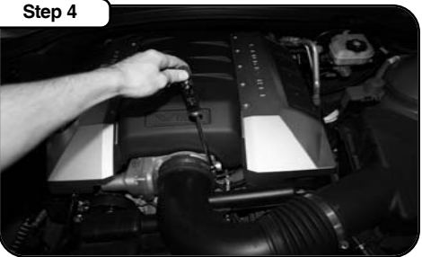
Loosen air intake tube clamp at throttle body inlet.
