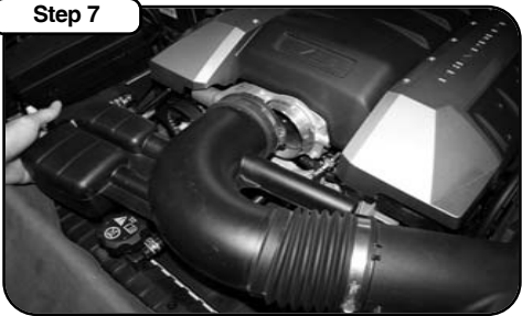
Disconnect air intake tube from throttle body.
