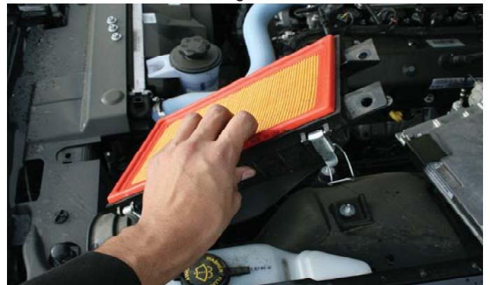
8- Remove the lower intake box from vehicle.
