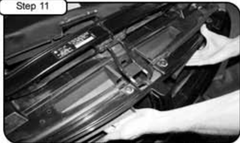
For easier installation, the next three steps will require an assistant. Have person A hold the scoops in position as shown. With BMW 320i, only the passenger side (p/n 05-01017) is installed.
