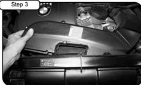
Pull back ram air duct and remove.
