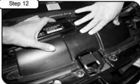
Have person B re-install the cover and secure with plastic pin clips that were removed earlier. (See steps 4-6)
