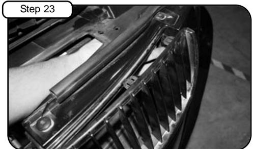
The grills are held in place with push clips. To remove, reach in behind each grill and push forward.
