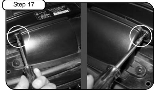
Remove screws on ram air duct using T25 torx bit. (Save for later installation)
