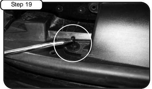
With flat head screwdriver, carefully pry and push up plastic pin.
