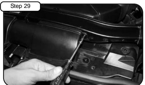
Re-position ram air duct from step 3. Secure using the 2 screws from step 17 and tighten using T25 torx bit.
