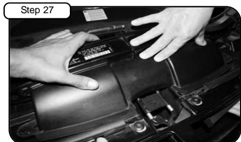
Have person B re-install the cover and secure with plastic pin clips that were removed earlier. (See steps 19-21)
