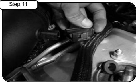
Re-connect air temp sensor harness.
