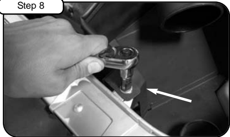
Tighten down housing using OE bolt. Use 10mm socket or wrench.
