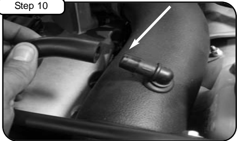
Re-connect crank case line to fitting on tube.
