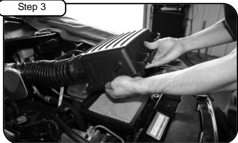
Disconnect air temp sensor and crank case line. Lift up and pull OE air box out of vehicle.
