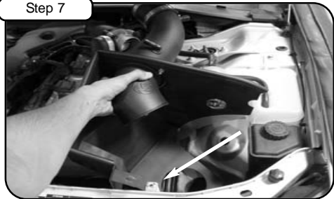
Install intake into vehicle. Position housing to tab.
