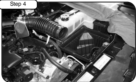
Loosen and remove OE intake tube with 5/16" nut driver. Remove bottom air box out of vehicle. Remove air temp sensor.
