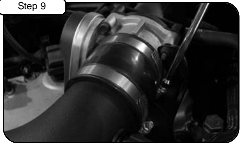
Tighten clamps using 5/16" nut driver.
