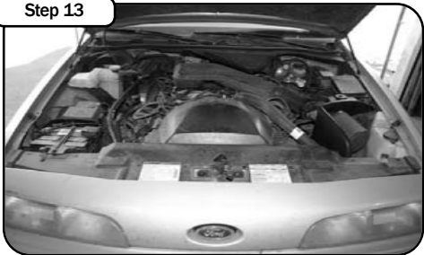
Place enclosed CARB EO sticker on a clean/smooth surface on or near the intake system. Your installation is now complete. Make sure you tighten all clamps/nuts and check all electrical connections. Re check periodically
