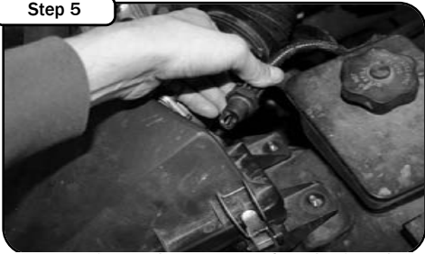
Remove the factory air temp sensor. Set aside for re-installation.
