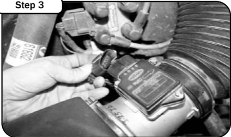
Disconnect MAF sensor. Using 5/16 nut driver, loosen intake hose and disconnect.
