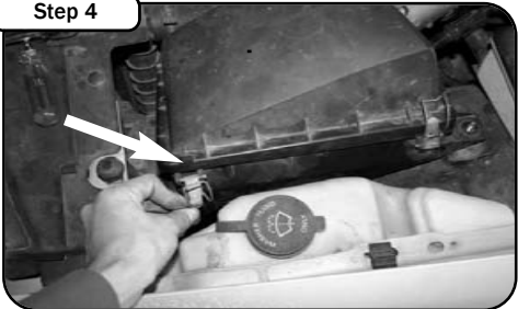
Unclamp the 2 factory airbox clips.
