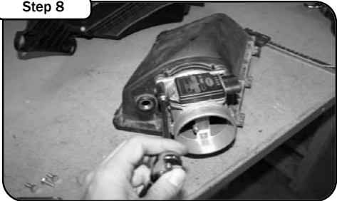
Using a 10mm socket, unscrew the 4 factory screws securing MAF sensor. Disconnect the MAF sensor and transfer onto new housing using new gasket provided.
