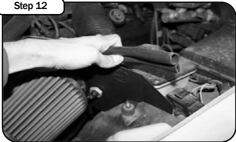
Install 7/16 trim seal provided on new housing.
