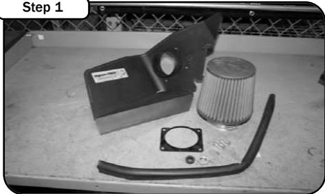
Complete kit. Make sure all components are present prior to beginning installation.
