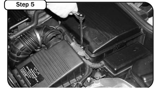
Remove the 10mm bolt that is located in the back of the air box securing the battery tray in place. Set the bolt to the side for later use.
