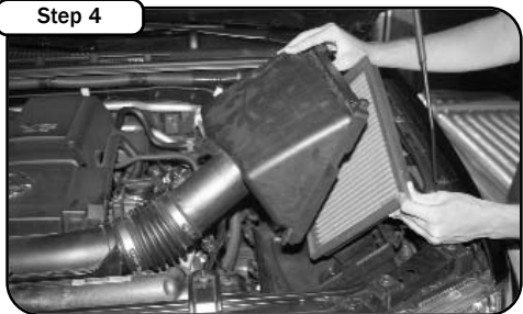
Remove the upper portion of the air box and the factory air filter.
