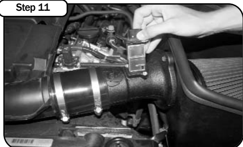
Transfer the MAF sensor to the aFe intake tube. Secure with the supplied gaskets, spacers, and screws. Make sure you pay attention to the direction of the arrow on the MAF sensor.
