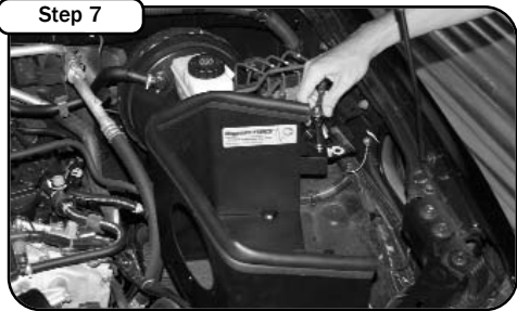
Place the rubber trim seal along the edge of the housing. Lower the housing into the engine bay secure housing with the bolt removed in step 5.
