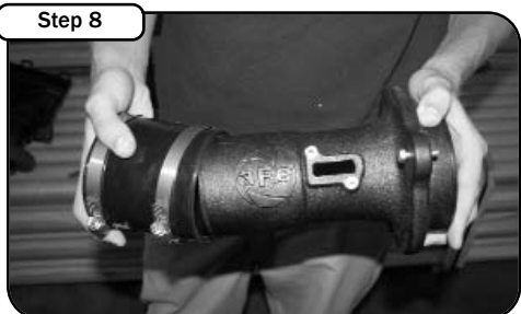
Place the coupler on to the intake tube. Do not tighten clamps at this time.
