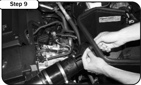
Slide the intake tube assembly into the housing . Secure the tube to the housing with the supplied M6 hardware. Tighten and secure the hose clamp.
