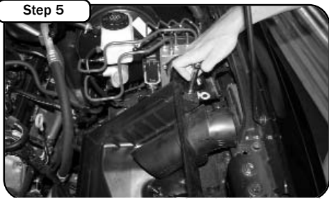
Remove the 10mm bolt on the side of the air box set aside for later use. Lift the lower air box up and out of the engine bay.
