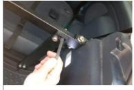
Rotate the vertical bars for attachment to the top bar. This may require the use of one Allen tool to line the holes up due to pretensioning of the
