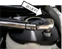
5) Center and align the Strut Tower Brace cross bar. Tighten all M7 Strut Tower Brace **bolts** to **35 ft-lbs** (47.5 Nm)
