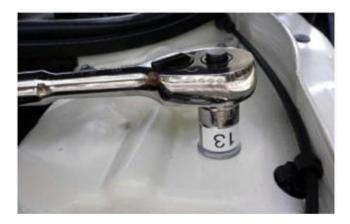
3) Using the 13mm socket, remove the 6 nuts at the top of the strut towers (3 on each side).
