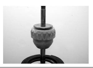
STEP 5 Slide the factory rubber bump stop over the strut piston. Slide the piston washer over the rubber bump stop.
