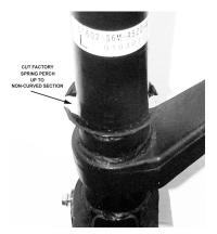
Once the front struts are removed, the factory spring perches can be trimmed in order to maximize the adjustment range of the coilovers. Trim the perches to the area where they no longer curve upward. There should be material left for the sleeves to sit squarely. Please use caution. DO NOT cut into strut.
