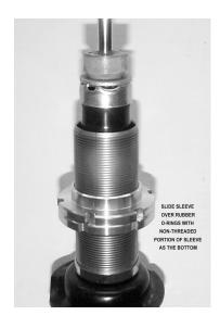
Slide (tall 115mm) threaded sleeves over the rubber O-rings. Make sure that the non-threaded portion of the sleeves are sitting squarely on factory spring perches. You may use lubricant (WD-40) to help slide the sleeve over the rubber O-rings more easily.
