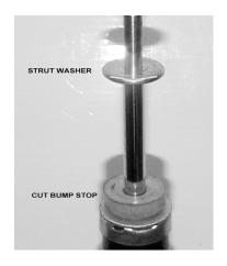
Slide the rubber o-rings (provided) over the struts. Each strut should use (2 rubber O-rings) to secure the top and bottom of the sleeve. Secure O-rings with electrical tape. Next, cut factory bump stop in half, using the larger half. Slide over strut pistons. Place strut washers over strut pistons.
