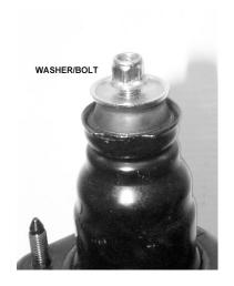
Place the correct coilover springs (0600-250-006) on to threaded sleeve perches. Then place the factory strut mounts over springs. Next secure them with washers and tighten with lock nuts. Install entire coilover assembly back in to suspension. Please refer to factory manual or equivalent. The factory dust covers will not be used.
