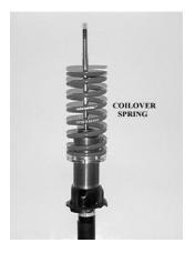
Place correct spring over sleeve and onto dual locking perches.
