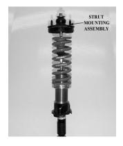
Place the strut mounting assembly back onto spring. Tighten self-locking nut. Re-install into vehicle. Adjust coilover height accordingly.
