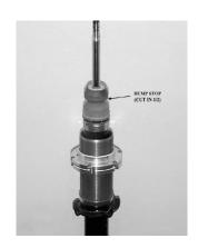
Each strut should use (2) o-rings to secure the top and bottom of the coilover sleeve. Choose the o-ring size that offers the securest fit. After properly positioning the o-rings, secure them by wrapping with duct/electrical tape. Some applications may not require the use of rubber o-rings.
