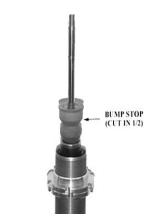
Slide tall (125mm) coilover sleeve over strut and o-rings, with the non-threaded portion of the sleeve as the bottom. If there is too much play between the strut and sleeve, thicker o-rings and/or tape will be needed. Properly installed o-rings will securely fit sleeve to strut. You may use a lubricant (WD-40) to help slide the sleeve over more easily.
