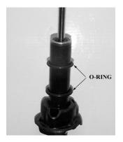
Place rubber o-rings onto strut. Each strut should use (2) o-rings to secure the top and bottom of the coilover sleeve. Choose the o-ring size that offers the securest fit. After properly positioning the o-rings, secure them by wrapping with duct/electrical tape. Some applications may not require the use of rubber o-rings. Notice the upside down spring perch.
