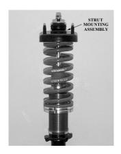
Place the strut mounting assembly back onto spring. Tighten self-locking nut. Re-install into vehicle. Adjust coilover height accordingly.
