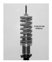
Place correct spring over sleeve and onto dual locking perches.
