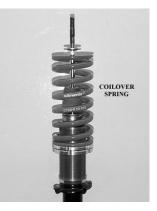
Place correct spring over sleeve and onto dual locking perches.
