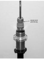
Each strut should use (2) o-rings to secure the top and bottom of the coilover sleeve. Choose the o-ring size that offers the securest fit. After properly positioning the o-rings, secure them by wrapping with duct/electrical tape. Some applications may not require the use of rubber o-rings.
