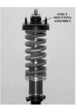
Place the strut mounting assembly back onto spring. Tighten self-locking nut. Re-install into vehicle. Adjust coilover height accordingly.
