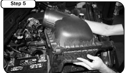
Loosen the 10mm nut at front of air box and remove. Carefully grab and pull out OE intake system from vehicle.
