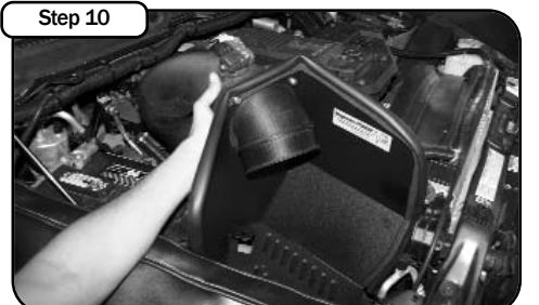
Install new housing with intake tube into vehicle. Position tube and housing to factory position.
