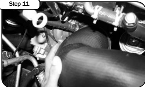
Make sure intake tube is inside of OE coupler. Do not tighten clamp at this time (see step 13).
