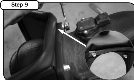
Install trim seal to housing, make sure cutout is at perm-nut on housing. Install tube to outside of housing. Tighten using hex screws, split and flat washers provided with 3/8" socket or wrench.
