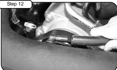
Install new 3/8" hose provided to valve cover side and new tube side.
