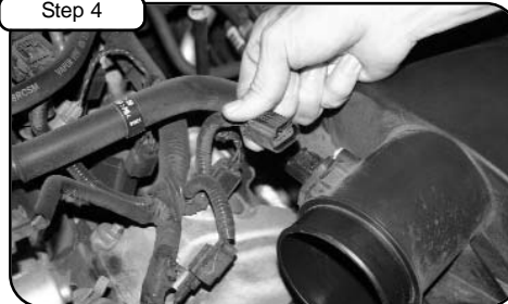
Disconnect MAF sensor harness.
