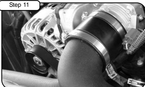
Tighten clamps with 5/16" nut driver.
