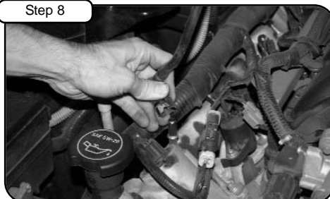
Remove factory crank case line from engine.
