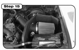
Place enclosed CARB EO sticker on a clean/smooth surface on or near the intake system. EO identification label is required in passing the Smog Check Inspection. Complete kit installed.
