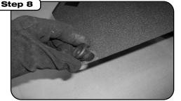
Place saved grommets into holes on the bottom of the aFe heat shield.
