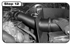
insert tube through heat shield so that the flange is on the inside of the heat shield and insert into coupler installed in previous step.
