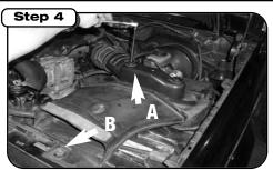
Using an extension from a 1/4" drive ratchet, fully loosen plastic bolts on top of factory air box (a), remove bolt securing front of air scoop to core support (b)
