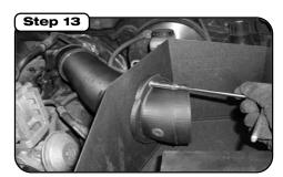
Using provided hardware, secure tube flange to heat shield. After tube has been secured to heat shield, tighten clamp holding the coupler to the
