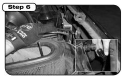
Using a 7/16" socket, remove nut securing lower air box half to engine compartment. Disconnect electrical harness going to temperature sensor on the side of the air box.
