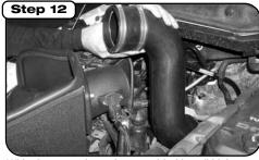
With clamps and couplers provided install high temp coupler at turbo side and 4"x3" urethane coupler at filter side, tighten using 5/16" nut driver. Install preoiled filter onto intake tube and tighten. Do not use any oil or grease when attaching filter. Reattach
