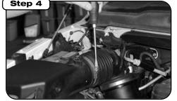
Loosen clamp holding factory tube to factory airbox and clamp at turbo. Remove complete system.
