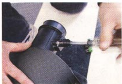
▲ At the outboard end, a single bolt secures the rectangular airbox to the inner fender. With this removed, the airbox/mass air assembly can be lifted out.
