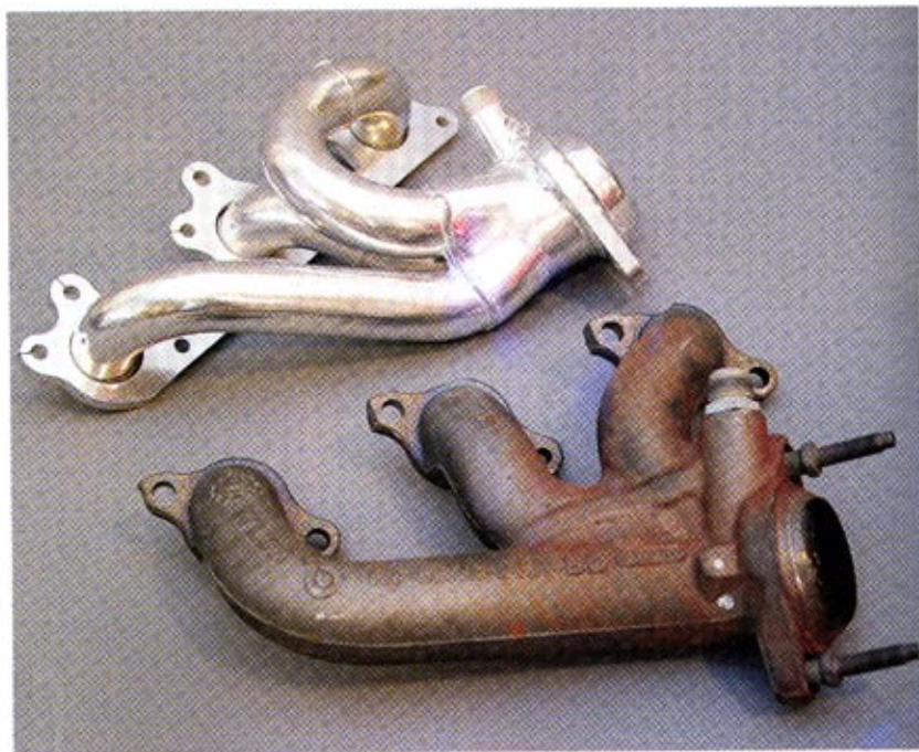
▲ The 4.0-liter V6 manifolds don't look all that restrictive, resembling the swoopy 427 FE cast-iron manifolds of the '60s. Looks can be deceiving however, as the JBA Cat4wards, with their 1.5-inch mandrel-bent primaries and proper collector design, provided surprising boosts in both horsepower and torque.
