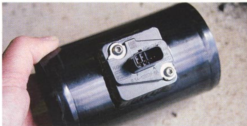
▼ When fitting the MAF wafer in the PHP inlet tube, be wary of the airflow-direction arrow visible here. Needless to say, if the MAF is installed backwards, good things won't result.
