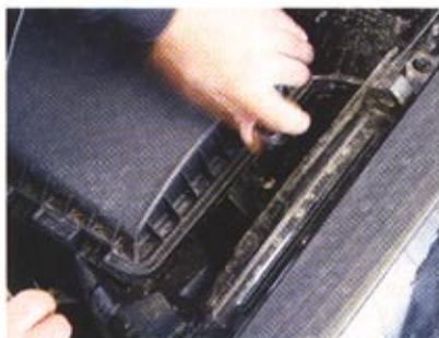
▲ At the outboard end, a single bolt secures the rectangular airbox to the inner fender. With this removed, the airbox/mass air assembly can be lifted out.
