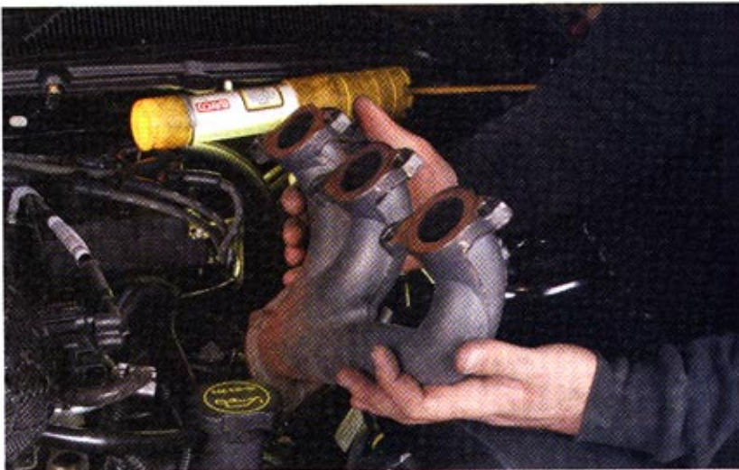
▲ There's sufficient working room around the exhaust manifolds that all six of their fasteners can be easily accessed from up top. JBA's instructions say to remove all manifold studs, and use the kit's bolts and lock washers to secure the headers. Though new ones are in the kit, Mike chose to reuse the factory steel manifold gaskets.
