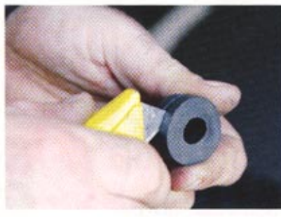
▲ Optionally, you can slice the stock airbox's rubber bushing and use the lower slim portion as an isolator when bolting the new filter assembly to the stock inner fender location. Don't try to use the bushing at full height, however, as the filter would mash up against the hood liner.
