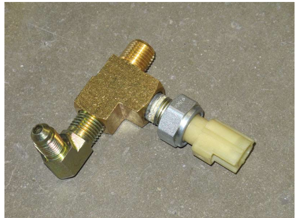
Fig. 13H: Oil Feed Assembly (shown removed for clarity)
