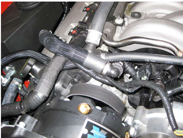
Fig. 5D-4: Modified Passenger Side PCV Hose, Installed
