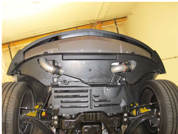
Fig. 12D-3: Plastic Undertray Trimming
