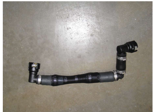
Fig. 5D-3: Modified Passenger Side PCV Hose
