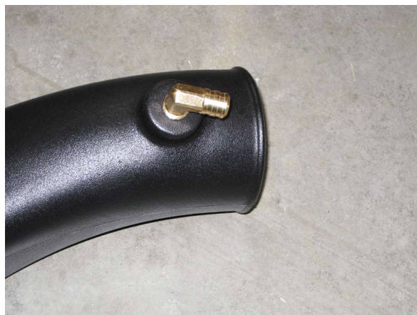
Fig. 11A: Air Inlet 3/8 NPT 90° Hose Barb Fitting
