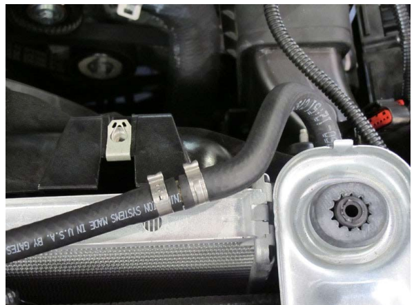
Fig. 3Y: Coolant Overflow Hose Cut & Splice
