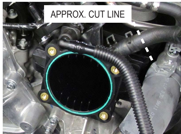
Fig. 8B-1: Cut Vacuum Hose (some components removed for clarity)
