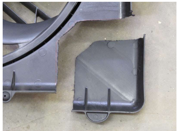
Fig. 3AE: Air Dam Location Cut
