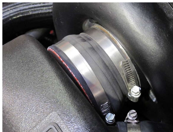
Fig. 11B: Air Inlet to Supercharger Connection
