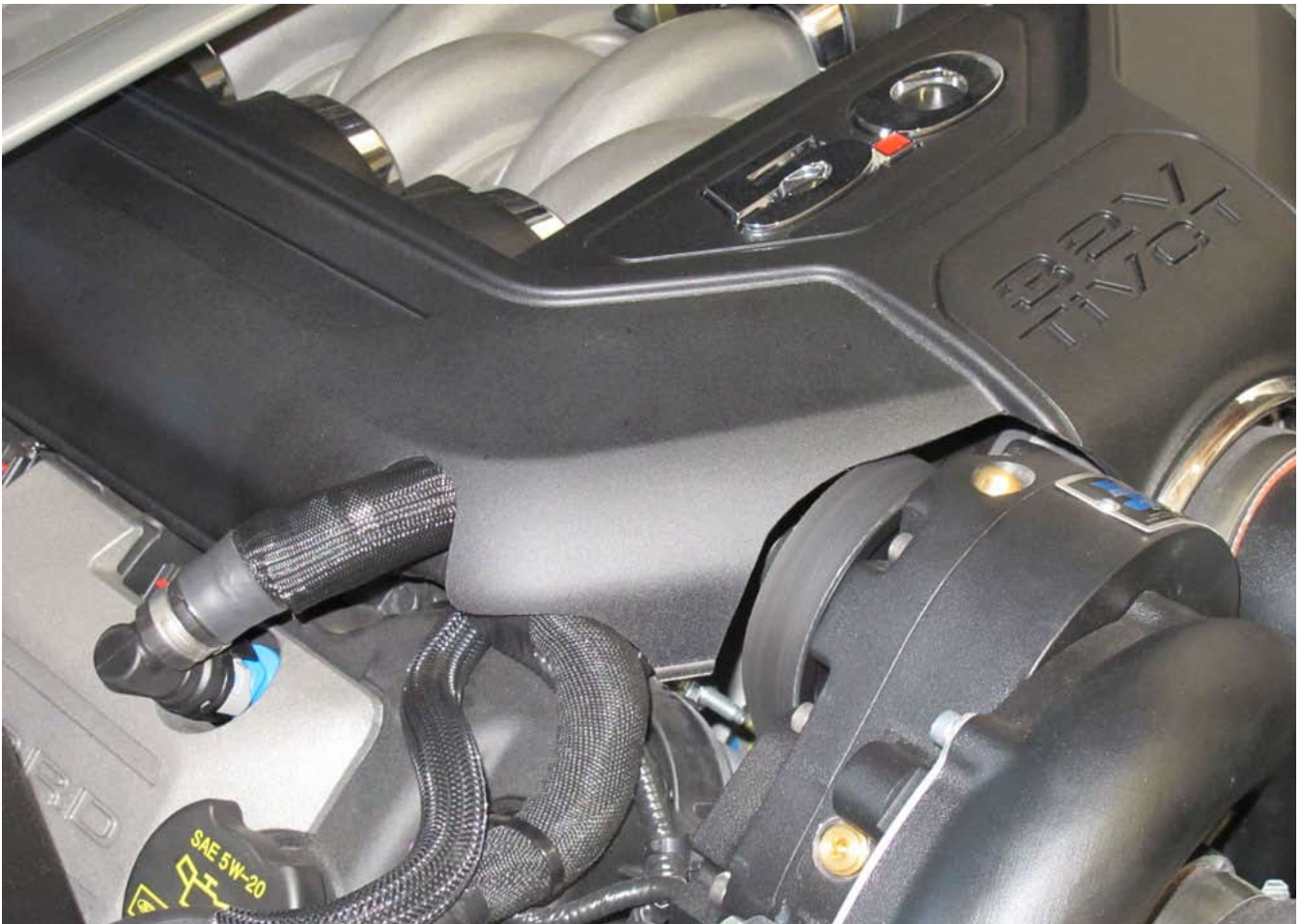
Fig. 10D-1: Engine Cover Cut Detail
