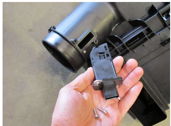
Fig. 1AD: MAF Insert (shown with OEM airbox removed)
