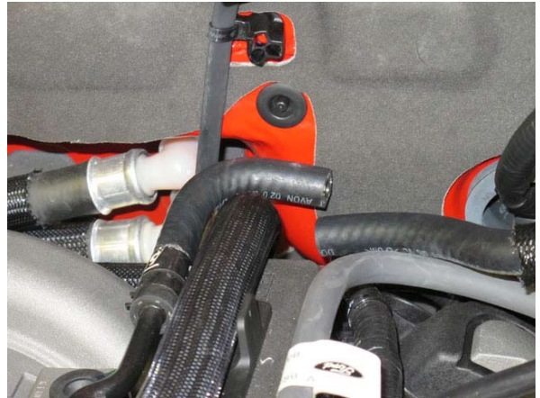
Fig. 8A-1: Vacuum Hose Cut
