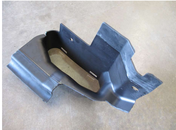
Fig. 12A-2: Modified Driver's Side Shroud
