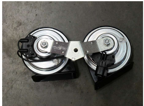
Fig. 6B: Modified Horn Bracket Orientation
