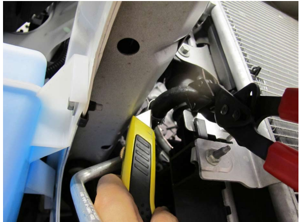
Fig. 2F: Clamping and Cutting A/T Hoses
