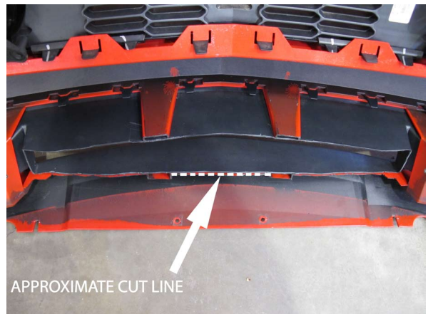
Fig. 12C-4: Bumper Cover, Center; Cut Line Reference
