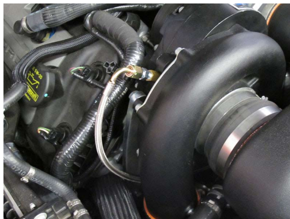
Fig. 13C: 90° Oil Feed Hose Installed
