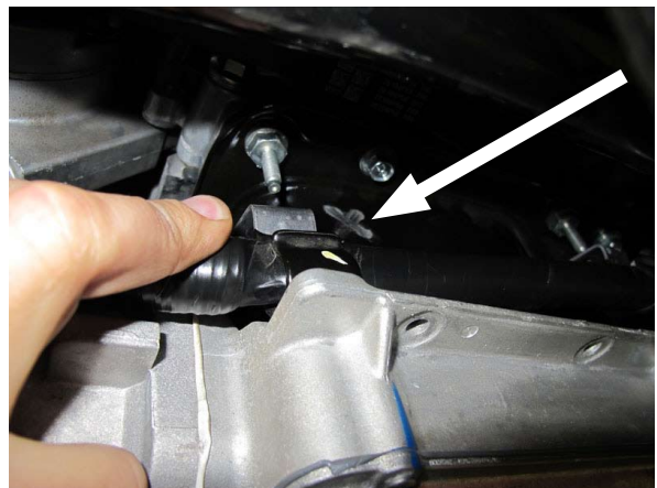
Fig. 14B: Oil Drain Fitting Installation Location
