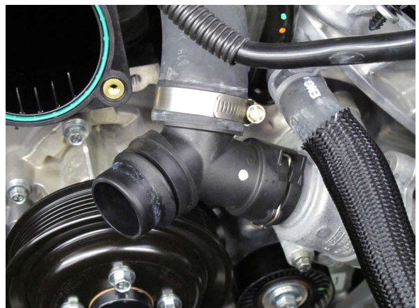
Fig. 2C: #28 Hose Clamp Orientation
