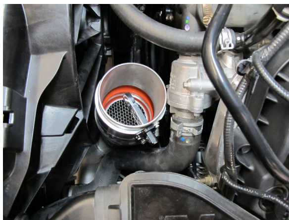
Fig. 7C-5: MAF Location (orientation will vary)
