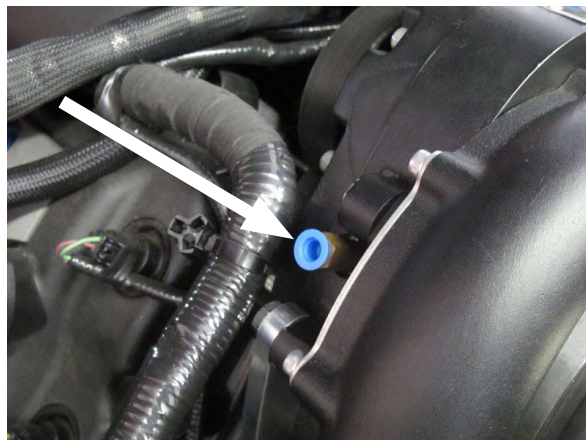
Fig. 13A: Supercharger Oil Feed Location
