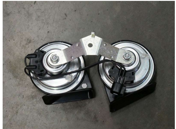
Fig. 6A: OEM Horn Bracket Orientation
