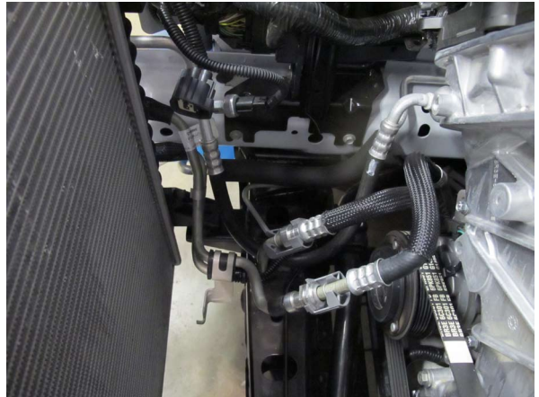
Fig. 2E: OEM A/T Cooler Hoses & Hard Lines
