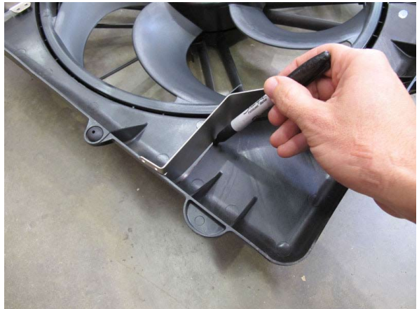
Fig. 3AD: Marking Air Dam Cut Lines
