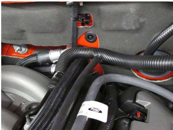
Fig. 8A-4: Vacuum Hose, Complete
