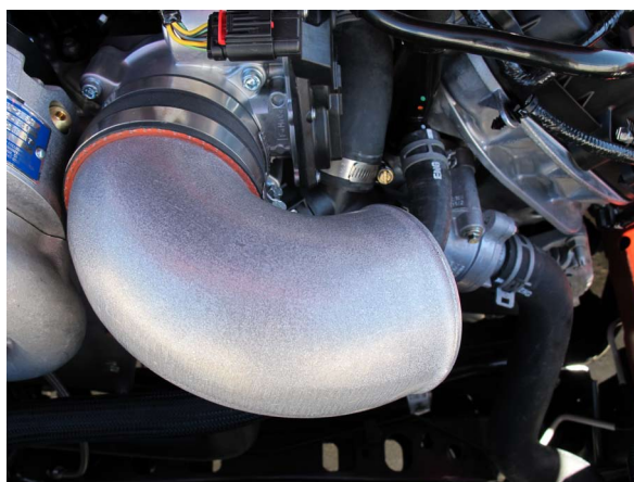
Fig. 7C-6: Ø3.5" x 120° Cast Aluminum Elbow
