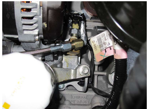
Fig. 13K: Oil Feed Assembly Orientation
