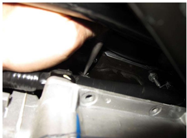
Fig. 14D: Punching Hole in Oil Pan
