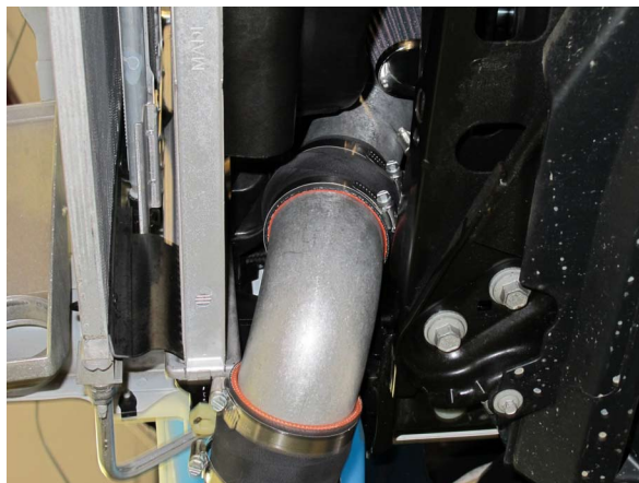
Fig. 7B-2: 90^\circ Tube and Bump Coupler
