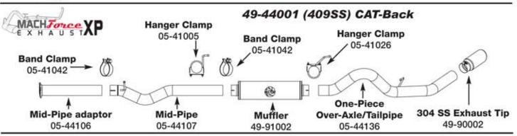
Step 1: (Read Instructions prior to installation) Remove your stock exhaust up to the cataytic converter from the rear of your truck working your way forward. It may be necessary to cut the pipes if the slip joints are stuck. Take caution not to damage the factory isolation mounts as they will be reused. Also save 4 nuts from the flange as they will be reused. It is recommended to not fully tighten the clamps until the entire system has been installed.
