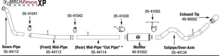
1: (Read Instructions prior to installation) Remove your stock exhaust from the rear of your truck working your way forward. Take caution not to damage the factory isolation mounts. If you want to remove the OE downpipe in one piece or without cutting, you must remove the transmission cross member and disconnect the dip-stick tube & sway bar end links. It is recommended to not fully tighten the clamps until the entire system has been installed.
