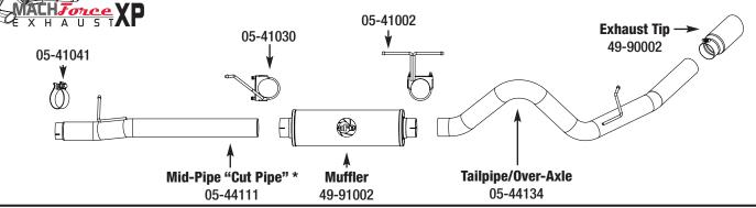
1: (Read Instructions prior to installation) Remove your stock exhaust up to the cataytic convertor, from the rear of your truck working your way forward. Take caution not to damage the factory isolation mounts. It is recommended to not fully tighten the clamps until the entire system has been installed.
