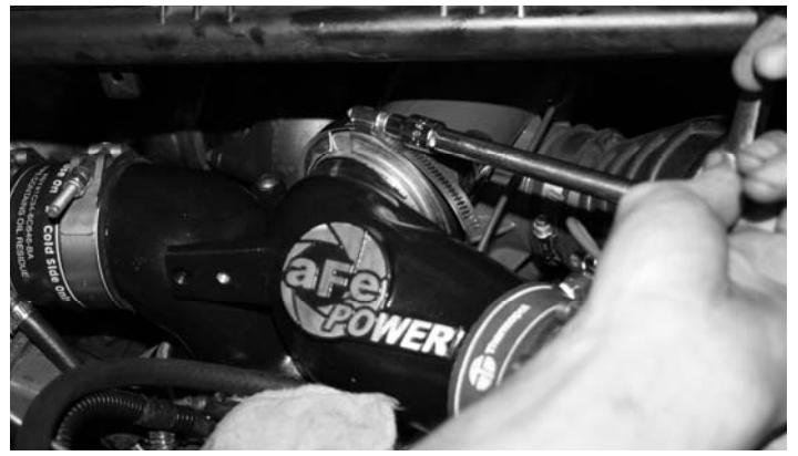
29- Once the manifold is in its desired position, firmly tighten down the turbo V-band clamp.
