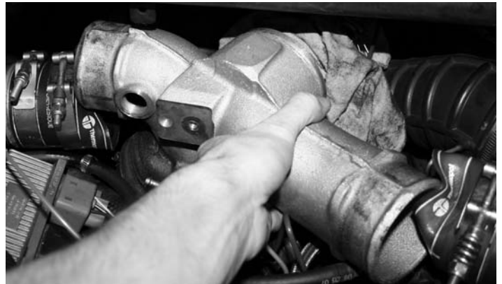
15- Pull the manifold out of the vehicle and be careful not to let anything fall into the plenum openings.
