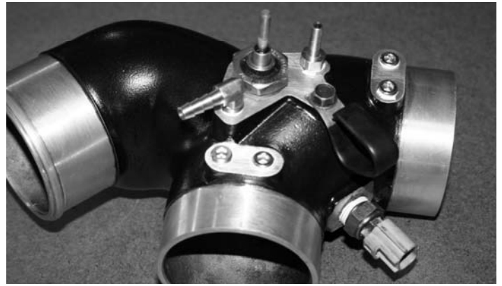
21- Install the heating element and temp sensor into the manifold and, last install the brass hose nipple. Torque all items to 16 Ft. Lbs.
