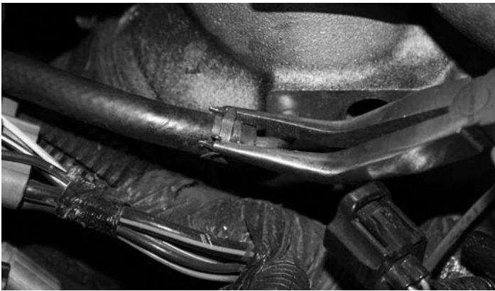
9- Using pliers to squeeze the clamp tabs, remove the rubber hose from the lower intake manifold fitting.
