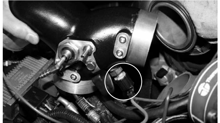
22- Connect the temp sensor before setting the manifold into the couplings.
