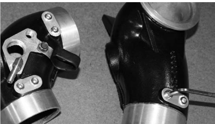
20- Install all 6 plugs and the 90 degree fitting elbow into the manifolds, then install the band clamp from the stock Y-inlet manifold.
