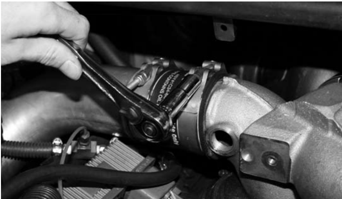
11- Loosen the clamp holding the manifold to the intercooler tube return side using a 7/16" deep socket.
