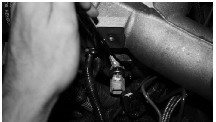
8- Remove the temp sensor from the lower manifold using a 13mm wrench and put aside for later install.
