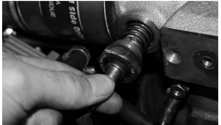
7- Once removed, put the heating element to the side for later install.
