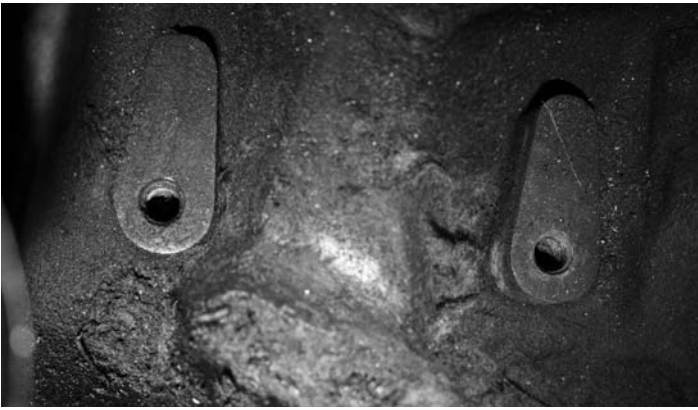
17- Use 3/8 - 16 tapped holes on the motor for the mounting support bracket.
