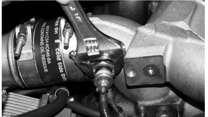
6- With an adjustable wrench, remove the heating element.
