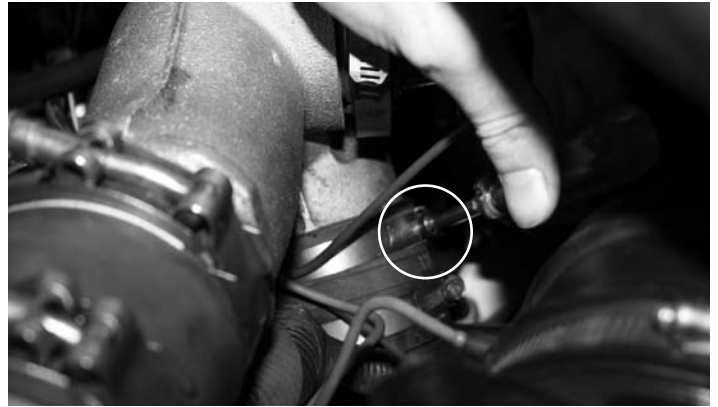
14- If needed, replace the couplings with Ford part number F81Z 6C640- FA available from your local dealer.
