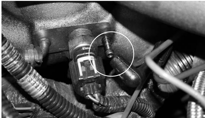
3- Disconnect the rubber boot/ hose.
