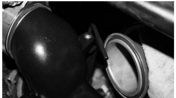
24- Line up the lower manifold with the support bracket and install the hex flange head screw supplied.
