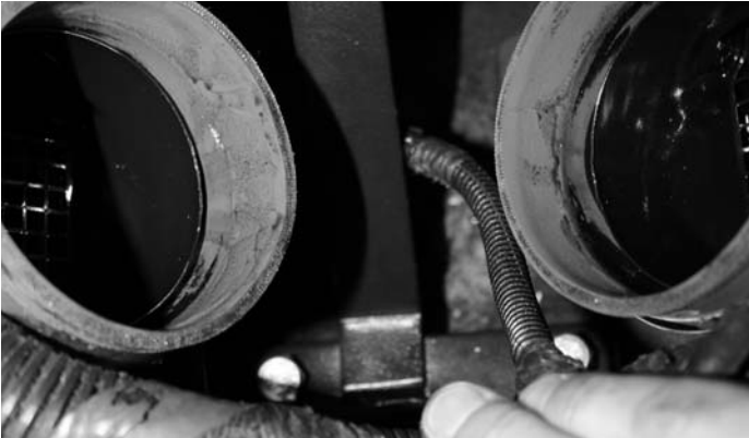
18- Install the manifold support bracket onto the top of the motor with 3/8 - 16 hex head cap screws supplied. Torque screws to 18 Ft. Lbs.
