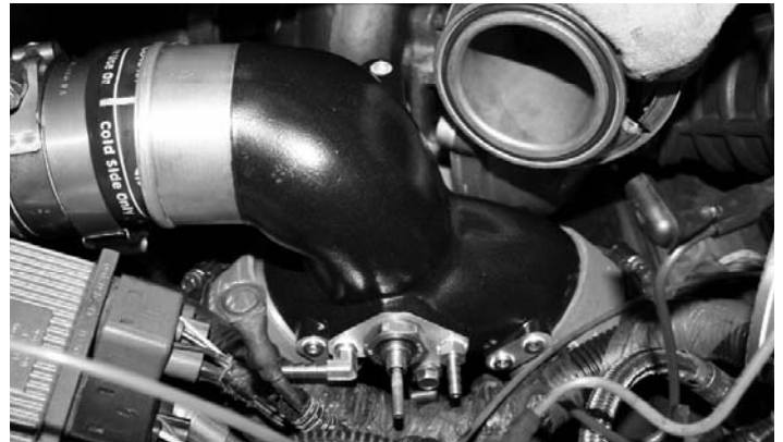
23- Once the manifold is in position, adjust the clamps to the desired location that makes them easiest to access.
