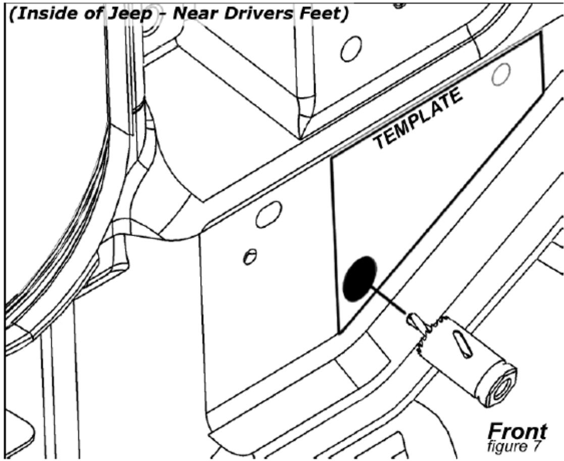
13. Using a 1" hole saw, cut the hole located in step 12.
