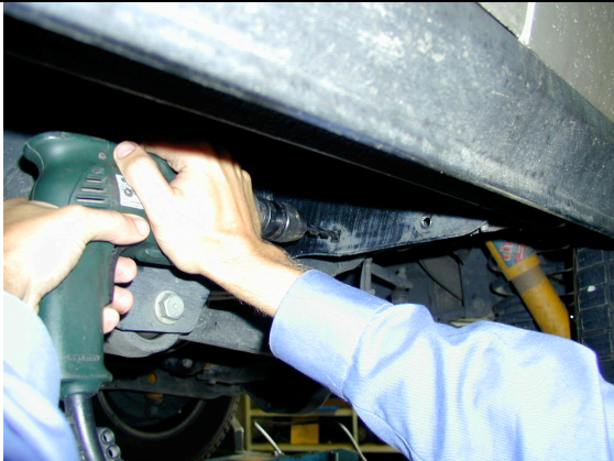
Drilling out rear body mount.
