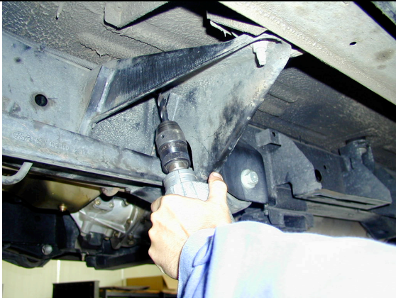
Drilling out front body mount
