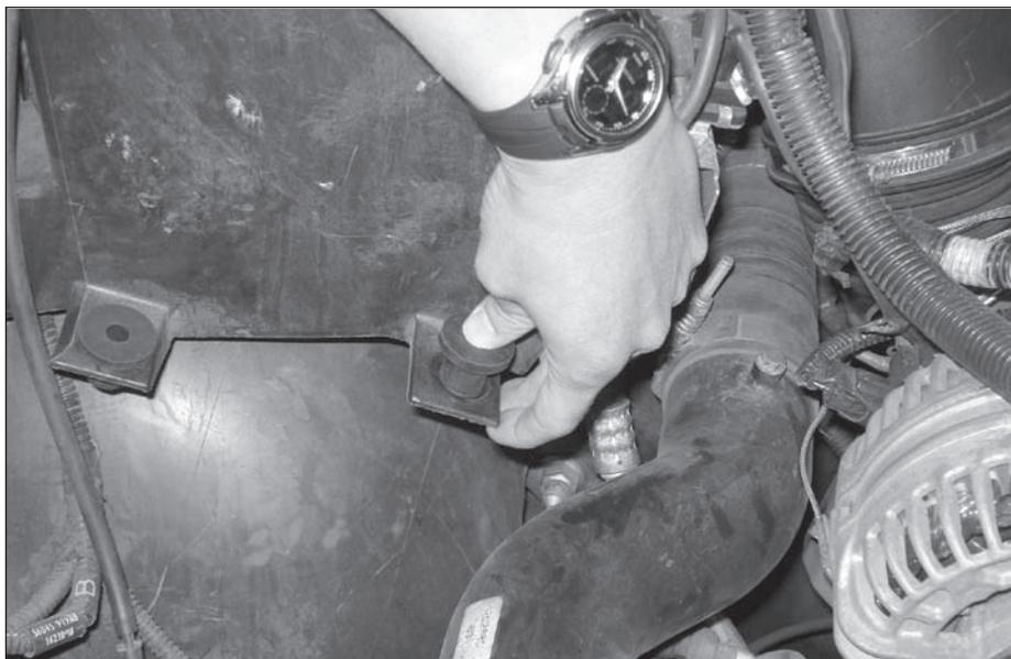
**7.** Install the supplied rubber Well-Nut as shown in **Figure 5**. Install flange side up, flush with bracket.
