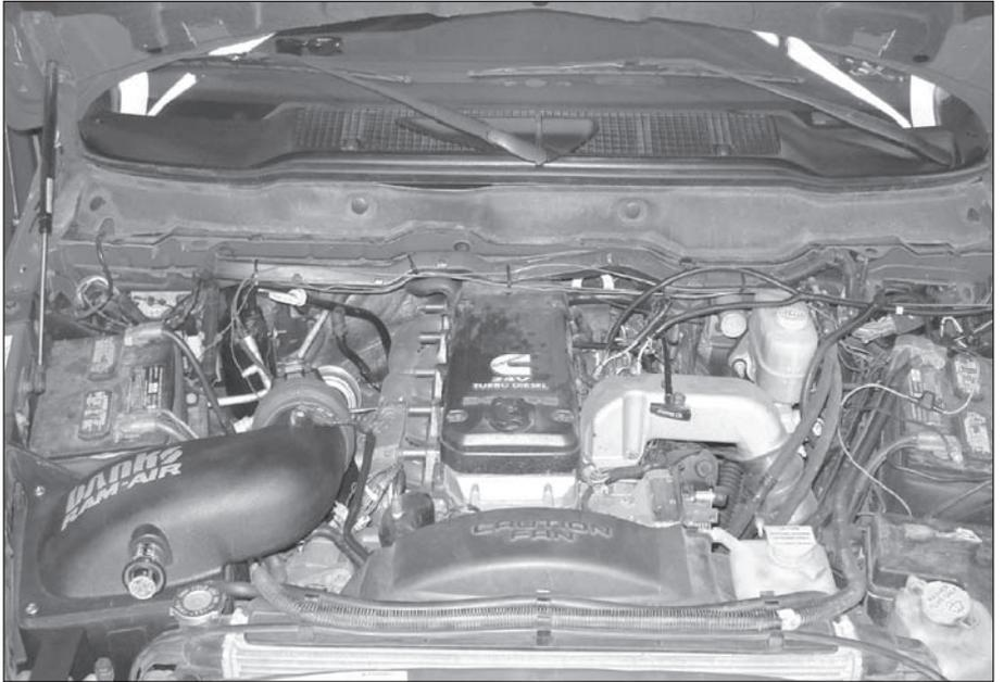
**25.** Install factory filter minder rubber grommet into the Banks cover. Insert the factory filter minder into rubber grommet.
