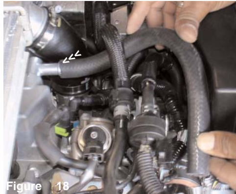
Figure 18 Press the 14"- 15mm breather hose over the vacuum port as shown above.
