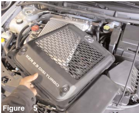
Figure 2 The two bolts are loosened and removed from the intercooler cover.
