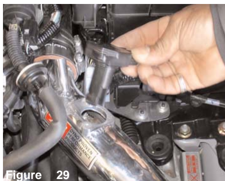
Figure 29 Prior to inserting the air mass sensor into the sensor adapter, moisten the O-ring with a light oil to prevent the O-ring from getting pinched.
