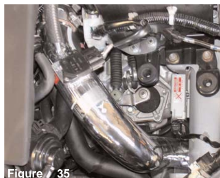
Figure 35 Align the entire intake for the best possible fit. Once you have cleared the intake from all moving parts, continue to tighten all nuts, bolts and clamps.
