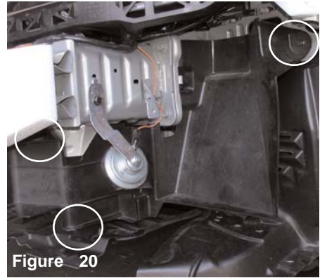
Figure 20 The splash guard inside of the driver side bumper is now removed. Loosen and remove three m6 bolts and 2 clips that holds the splash guard in place.
