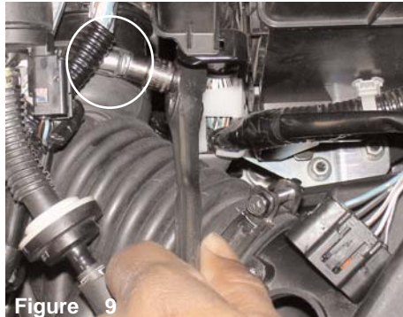
Figure 6 Remove the electrical harness clip from the air mass sensor as shown above.
