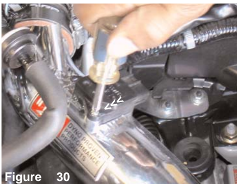
Figure 30 Once you have pressed the mass air flow sensor into the sensor adapter, use the stock screws to secure the sensor to the adapter.
