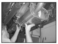
8. Insert the JBA intermediate pipe (A) hangers into the (2) rubber isolators then bolt the intermediate pipe to the factory catalytic converter assembly using the factory hardware.
