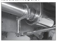
14. Support muffler and align straight up and down. Install 2 1/4" clamp (D) over 2-1/4î front muffler slip joint and tighten completely using a 9/16" deep wall socket. NOTE: Use anti seize on threads of clamps. See Notes #2.
