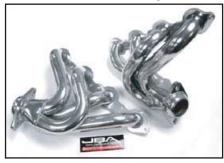
Get 20+hp and faster ET's with a set of smog legal stainless steel JBA Cat4ward® headers. Part No. Applicaton 1809S 04-06 Stainless 1809SJS 04-06 Silver ceramic 1809SJT 04-06 Titanium Ceramic
