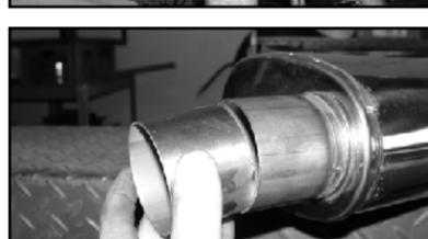
12. Install the new mufflers (A) with the offset end toward the front of the vehicle. See the picture above. If installing on the a 1500 HD you will need to insert the reducer bushing into the offset end of the new mufflers.
