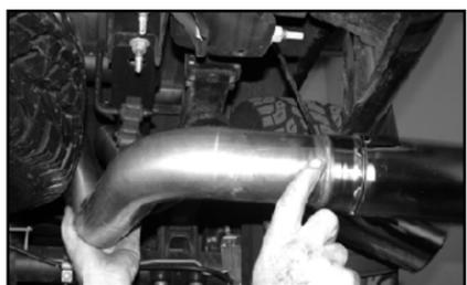
10. Insert turn out (C) and attach to turn out (D) using the supplied nut and bolt. Snug (C) and (D) together but don't fully tighten yet.
