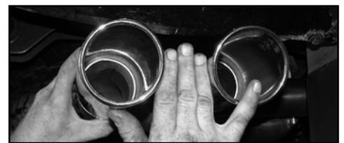
17. Align the tips on the turn outs (C) and (D) for proper clearance.
