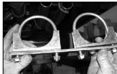
13. Assemble the new rear exhaust support bracket (G) with the supplied 3" clamps (F) as shown.
