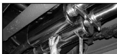
15. Tack weld the mufflers in place at the slip connections with the factory exhaust.
