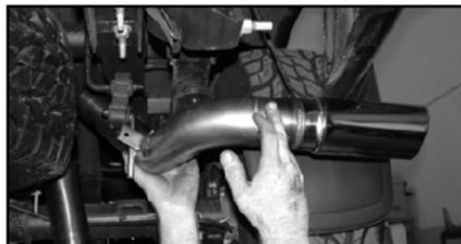
9. Take the turn out with hanger (D) and insert the hanger into the rear rubber grommet.
