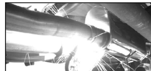
19. With the new exhaust system properly aligned weld the muffler into place.
