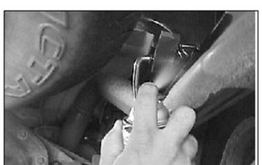
5. Spray lubricant on the rubber exhaust grommets behind the muffler.
