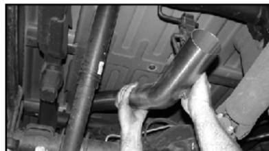
8. Pass the new JBA tail pipe (B) over the axle and insert the hanger into the forward rubber grommet.
