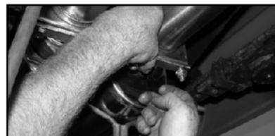
14. Position the assembled bracket at the rear of the mufflers over the slip connection with the tail pipes (B) and (E). Then align the mufflers.
