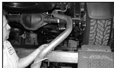
7. From the rear of the vehicle, remove the tail pipe assembly from the truck.
