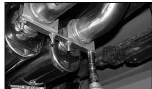
20. Finally tighten the support bracket.
