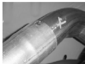
9. Install the supplied 2.5" clamps (C) over the muffler and intermediate pipe slip connection
