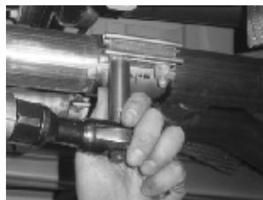
11. Check for proper alignment and adequate clearance around the new JBA tips. Tight all clamps
