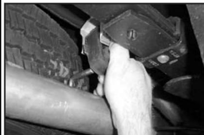
15. Install clamp (D) onto rear of muffler (#).
