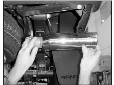
17. After installation, it is recommended that all clamps be re-tightened.
