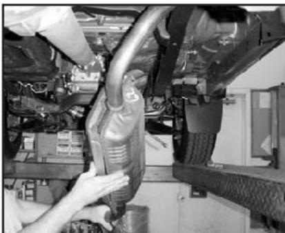
6. Remove the original exhaust system from the vehicle.
