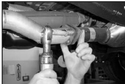
8. Tighten the fasteners.
