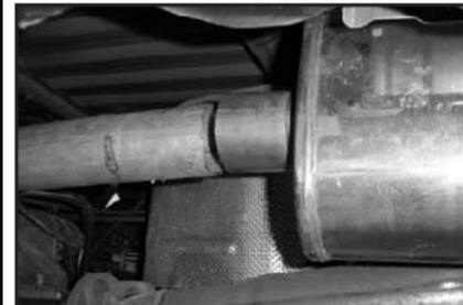
14. Install tail pipe hanger into factory rubber isolator.
