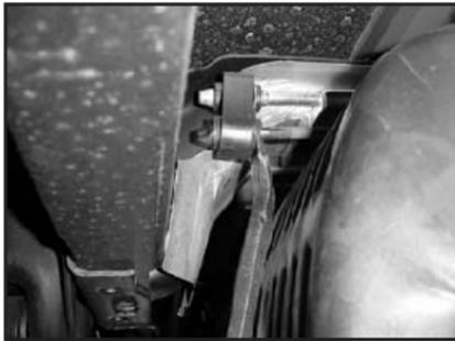
4. Using a pry bar or a pair of channel lock pliers remove hangers from rubber isolators at the top of the muffler.
