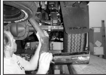
13. Insert tailpipe (C) into muffler (B).
