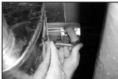
10. Insert hanger rods on the muffler into the factory rubber isolators.
