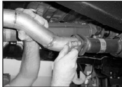
7. Using original fasteners, connect intermediate pipe (A) to the factory catalytic converter pipe.
