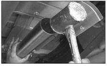
9. Install head pipe (A), aligning notch with locating pin. You may have to tap it on using a rubber mallet.
