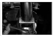
17. With tail pipe properly aligned, tighten rear muffler clamp/hanger (G) completely with 9/16" deep wall socket. NOTE: Use anti-seize on all threads of clamp. See note #2.
