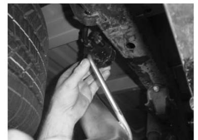
19. Insert turnout w/ tip and hanger into rubber isolator at the rear of the vehicle, near the spare tire.
