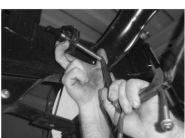
11. Install muffer hanger clamp (E) into rubber isolators near the rear of the factory muffler location.
