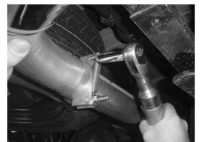
21. Align exhaust tip (D) properly and tighten clamp (G).
