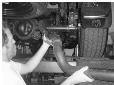
7. Remove tail pipe from the rear of the vehicle.
