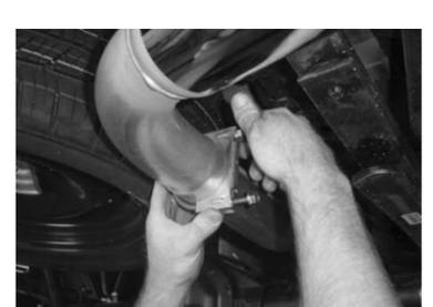
20. Position exhaust clamp (H) over slip connection on turnout w/ tip (D).
