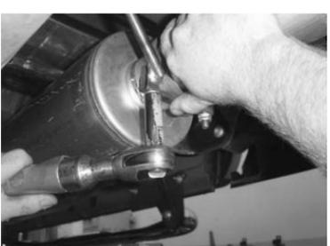
16. Align tail pipe (C) properly and tighten muffler hanger clamp (E).
