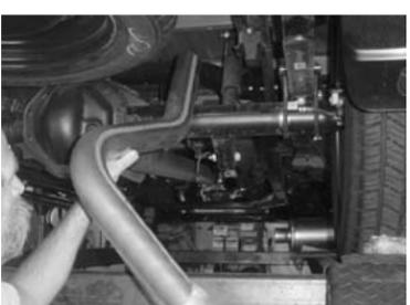
14. Install tail pipe (C) through the rear of the vehicle.
