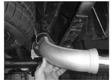
18. Install turnout w/ tip (D) at the end of tail pipe (C).
