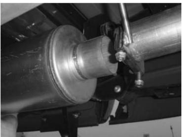
15. Insert tail pipe (C) through muffler hanger clamp (E) and into muffler (B).
