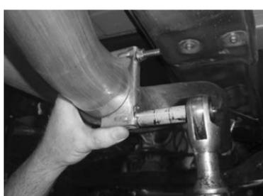
12. Install intermediate pipe (A) and secure with exhaust clamp (G).
