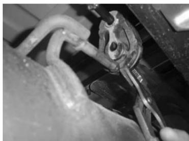
9. Remove muffer hangers from rubber isolators.
