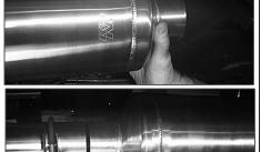
12. With JBA logo facing rear of vehicle, install muffler (B) over head pipe (A) making sure muffler bottoms out on slip joint.
