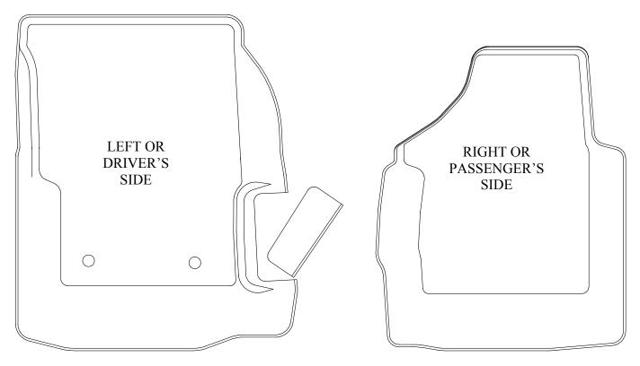
IF YOUR SUPER DUTY IS EQUIPPED WITH A MANUAL TRANSFER CASE SHIFTER, YOU WILL NEED TO TRIM YOUR LINER AS TO ALLOW IT TO FIT AROUND THE SHIFTER. TO TRIM, REMOVE THE MATERIAL FROM THE LOWERED AREA ON YOUR LINER AS DEMONSTRATED ABOVE. USE THE EDGE OF THE LOWERED AREA AS YOUR GUIDE. A PHOTO OF THE TRIMMED LINER IS SHOWN ON THE BACK OF THIS PAGE. A UTILITY KNIFE OR HEAVY SHEARS WORK WELL FOR TRIMMING.
