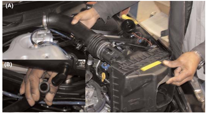
The entire air intake box, duct and sensor housing is removed in one piece(A). Before removing the air intake box from the engine compartment, disconnect the breather line connected to the box and crankcase (B).
