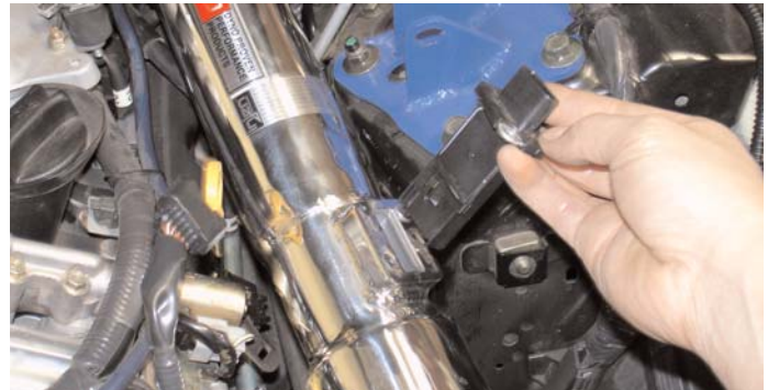
Press the stock MAF sensor into the machined adapter welded to the intake and use the stock screws to secure the sensor in place.
