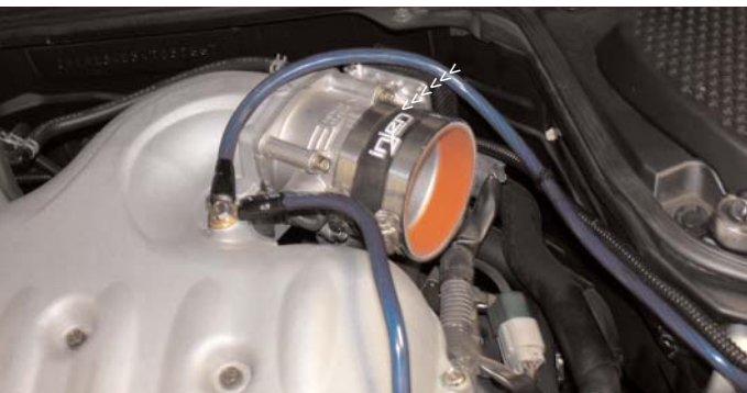
Press the 3 1/8" straight hose over the throttle body and use two medium .048 clamps, tighten the clamp on the throttle body at this point.
