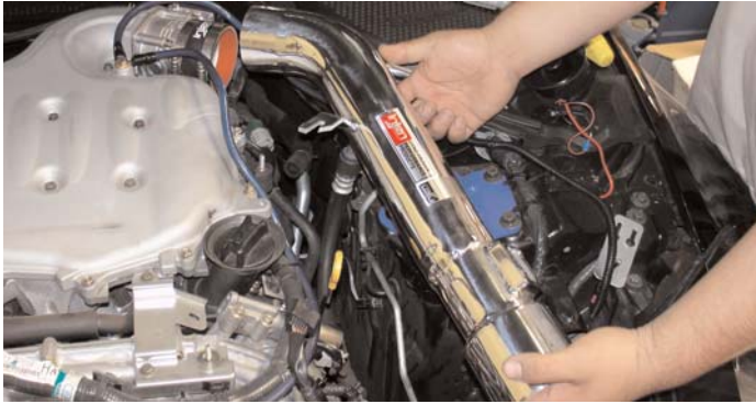
The crankcase breather line is attached to the intake port and the stock clamp is used to secure the line in place.
