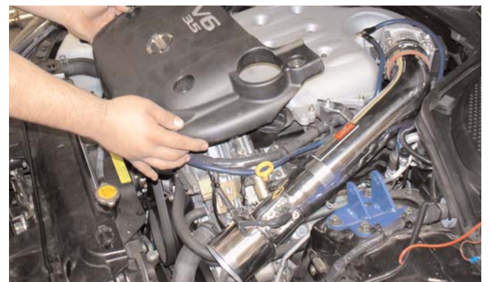
Once the entire intake is aligned and secured in place the intake manifold cover is re-attached.
