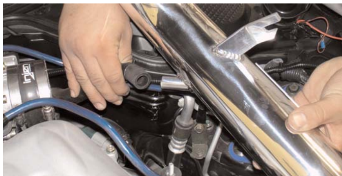
Take the primary intake and position it in place. The first step is to press the crankcase breather hose over the 5/8" port on the intake. Continue to align the entire intake by following the next steps of the instructions.
