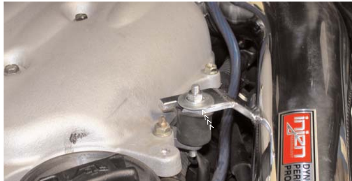
Once the intake is aligned use the m6 flange nut and fender washer to secure the intake in place.
