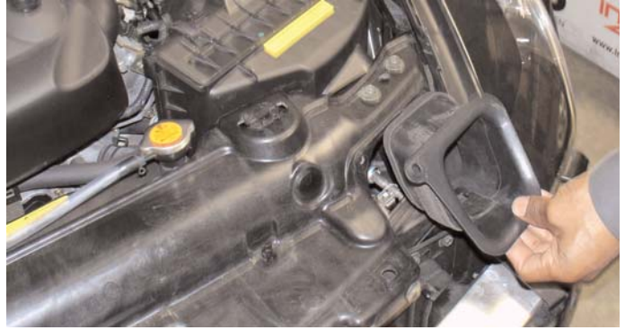
The front air scoop is removed in order to make room for the silicone intake hose.
