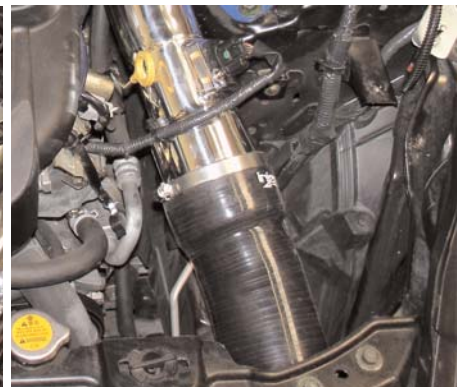
The 3 1/2" top end of the hose is pressed over the primary end of the intake. Use one of the large clamps to secure the hose in place.
