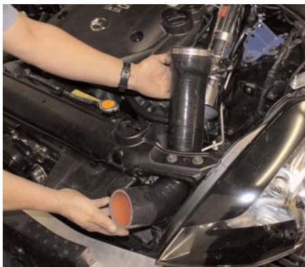
Slip the secondary silicone into the air scoop opening and point the front end down towards the front of the radiator.
