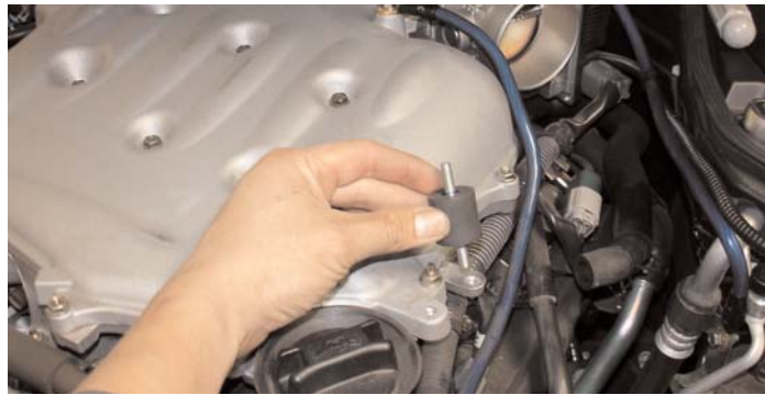
Screw the vibra-mount into the pre-tapped mounting point of the intake manifold. Screw the vibra-mount in until it is firmly in place.
