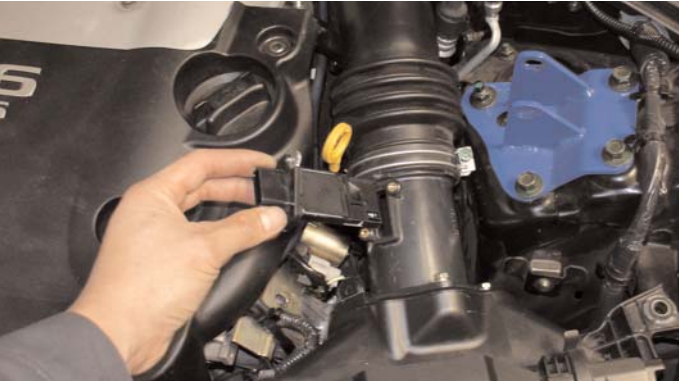
Remove the MAF sensor from the sensor housing. The sensor housing will no longer be used in this application.
