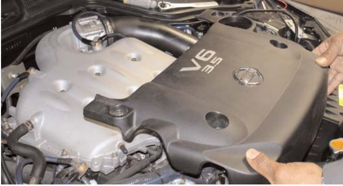
Remove the plastic intake manifold cover before installing the intake.
