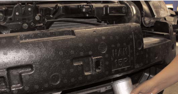
Prior to installing the cold air intake the front bumper will need to be removed. See next page diagram (A) for instructions.
