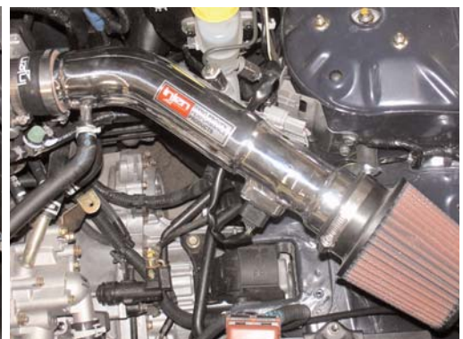
The installation of the short ram intake system is now complete.
