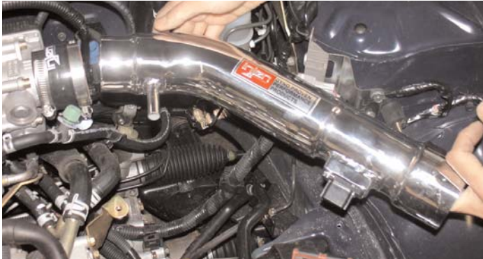
Take the assembled air intake and press the top section into the throttle body hose as shown above. While the top section is pressed into the throttle body hose the intake bracket is aligned to the vibra-mount stud.
