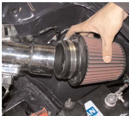
Short Ram installation: Take the filter and press it over the end of the primary intake. Once the intake is butted up against the filter stop continue to tighten the filter clamp.
