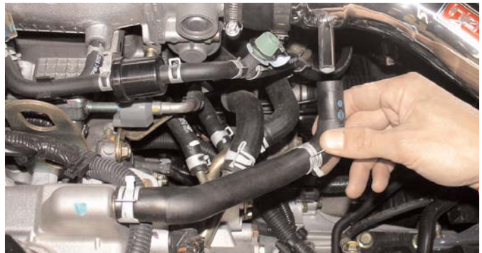
Press the stock crankcase hose over the 5/8" intake port and use the stock clamp to secure the hose in place.
