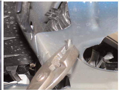
Take a pair of pliers and compress the plastic clip that holds the harness line in place. Compress and pull upward in order to remove the plastic clip.
