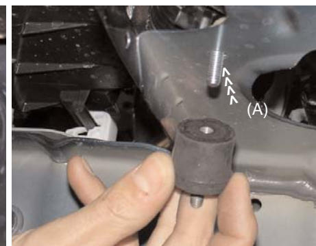
The m6 x 12mm bolt is inserted and is now protruding through the sheet metal. A male/female vibra-mount is attached to the m6 12mm bolt as shown above.
