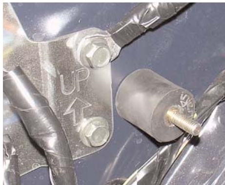
The vibra-mount has been screwed into the side wall of the strut tower mount. Turn the vibra-mount until the bottom butts up against the side wall.
