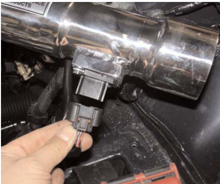
Take the harness clip and press it over the air sensor until you hear them snap in place. The snapping insures that you have good contact. page 3 of Part# SP1967
