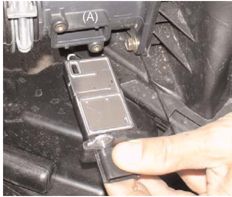
Remove the two screws from the sensor pad (A) and carefully remove the air sensor from the sensor housing as shown above.
