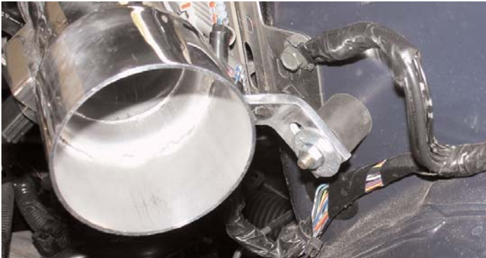
The m6 flange nut and fender washer is used to secure the intake to the vibra-mount stud. Do not over tighten the flange nut until the entire intake system has been installed and aligned.
