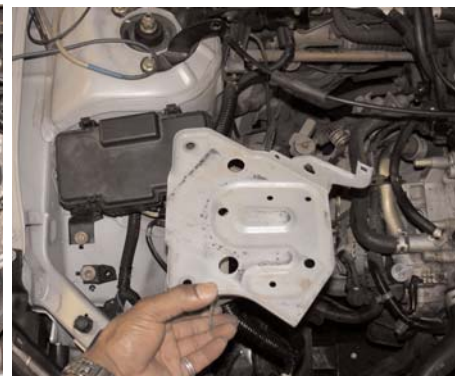
Once the battery has been removed continue to remove the plastic and metal battery tray.
