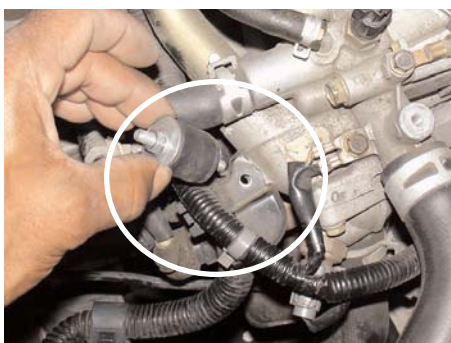
Screw the second vibra-mount into the brace next to the thermostat housing
