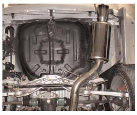
The new SES1898TT is finally here. A full 76mm slip-fit straight through, featuring a Titanium tip with an embossed Injen logo. This system when used with the test pipe already included in this kit delivers up to 25 h/p to the wheels.
