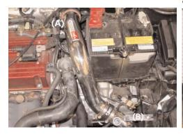
Hardpipe (B) connects to the driver side end tank outlet and to hard pipe (A). The stock rubber elbow is used on both sides of the tank.
