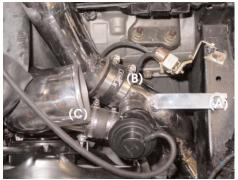
Top view of the bracket (A), blow-off valve (B) and cast intake (C) all connected and ready for the next step.
