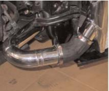
Here is a good shot of the 2 3/4" end inserted into the stock elbow located on the intercooler tank. Two .312 Power-Bands are used to secure the hard-pipes in place.
