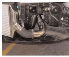
Here is a shot of hardpipe (B) connected to the stock hose on the intercooler tanks. Use two .312 Powerbands to connect hardpipe (B) to intercooler end tank.
