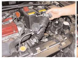
Remove the stock air intake duct connected to the turbo outlet (A) and the air intake box (B). This system must be used with an up graded intake system. This system cannot be used with the stock air intake system.
