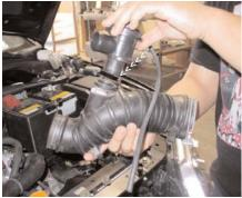
Remove the blow-off valve from the stock intake
