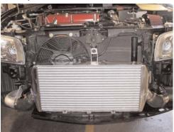
This large heavy 23" x 11 1/2" x 3" intercooler will fit the stock piping and elbows or Injens intake system. Intercooler cores are made in Australia. This intercooler will support up to 750 h/p
