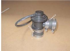
Press the new reinforced short hose over each port on the blow-off valve. Use the .024 mini clamps provided in this kit to secure the hose in place.
