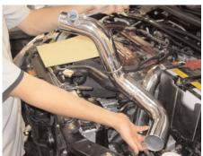
Take the secondary hardpipe and lower it into the bumper section. Insert the lower end into the stock hose on the intercooler port but do not tighten the two .312 Power-bands that are to be
