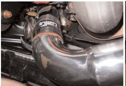
Press the 2" straight hose over the turbo inlet, use two .262 Powere-bands. Set one end of the hard pipe into the turbo intlet and press the other end into the stock elbow, use two .312 Power-bands on the end tank side.
