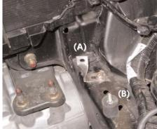
Take the small 1450T bracket and mount it to the held the air intake box and boost solenoid in place. frame of the car, use the stock bolt to secure the bracket in place(A). Screw the vibra-mount into the pre-tapped hole on the same frame as the bracket(B).
