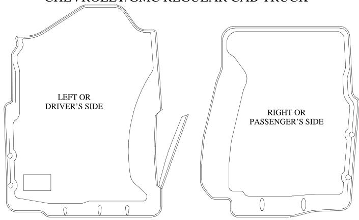
IF YOUR VEHICLE IS EQUIPPED WITH A MANUAL TRANSFER CASE SHIFTER, YOU WILL NEED TO TRIM YOUR LINER AS SHOWN ABOVE. TRIM DOWN THE EDGES FORMED BY THE RECESSED AREA ALONG THE WALL AND ACROSS THE SCRIBED LINE. YOUR LINER WILL NOW FIT AROUND THE TRANSFER CASE SHIFTER HOUSING. A UTILITY KNIFE OR HEAVY SCISSORS WORKS WELL FOR TRIMMING YOUR LINER.
