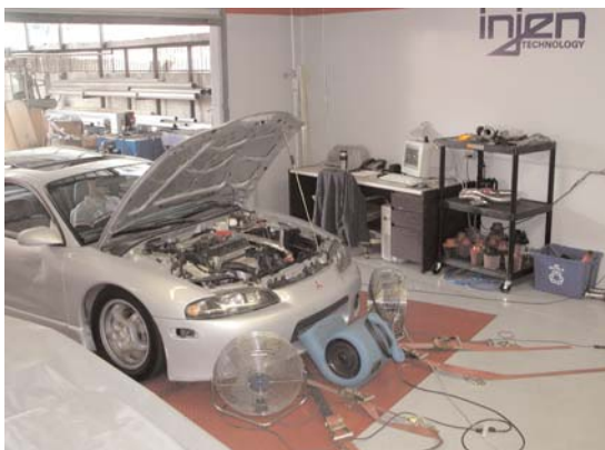
Injen Research and Development Team at work testing various intake tubing and filters. Top end showed an 8.8 horse power gain.
