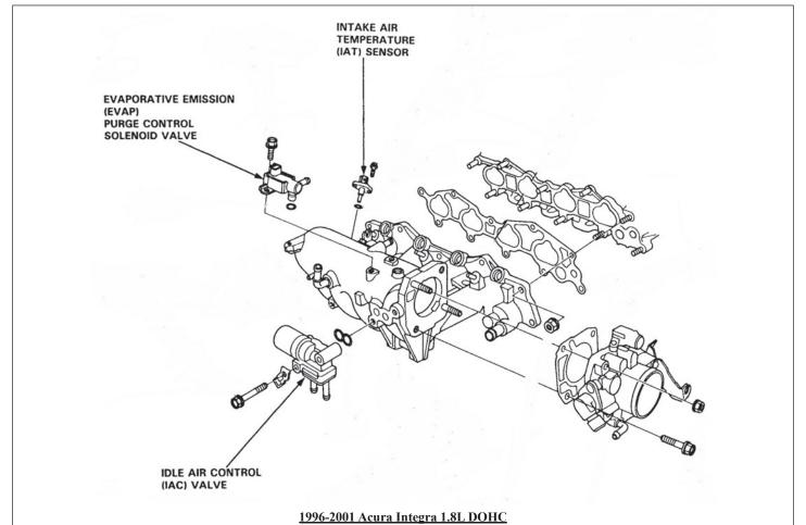
A T-fitting will be used to connect the PCV hose and the EVAP hose onto the larger vacuum stem located on the manifold body. The other EVAP hose will be connected back to the charcoal canister. Due to the manifold design, it is recommended that the EVAP unit be zip-tied to a secure location.
