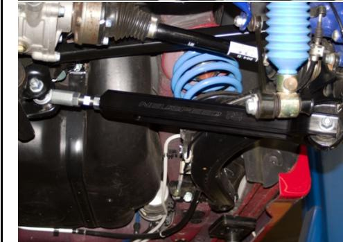
6. Using a floor jack and a block of wood under cast trailing arm, raise jack to preload the suspension. Torque all control arm bolts to 70Nm (52 ft/lbs). that were either loosened or removed.
