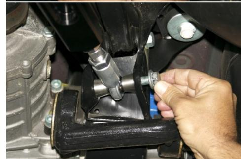
4. **Note:** For extreme conditions, optional ball-joint protection boots are available, part number 32.10.70. If purchased, install boots on ball-joints now. Install the NEUSPEED Adjustable Control Arms using the supplied outer M12 x 80mm bolt, washer and original nut, then install supplied stainless steel ball joint spacers and the original inner M12 x 80mm bolt and nut.
