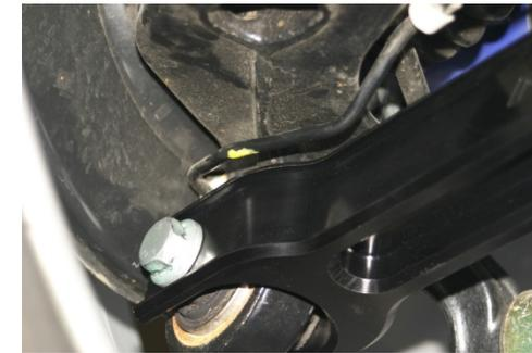
5. Check for ample clearance between brake line and control arm.
