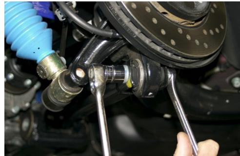
3. Remove the inner and outer control arm bolts using an 18mm wrench and 18mm socket.
