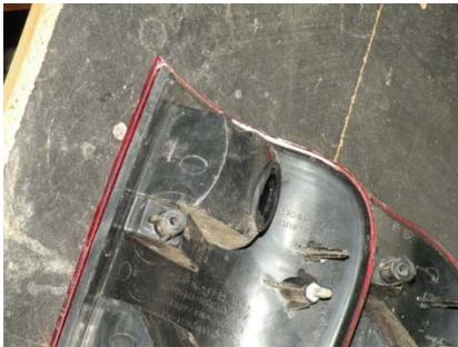
**\*\*\* You Are Required To Have At Least 1" of Room Around All Sides Of The Strobe Element. Failure To Leave Room May Cause Fire or Severe Damage To Components During Operation. \*\*\***
