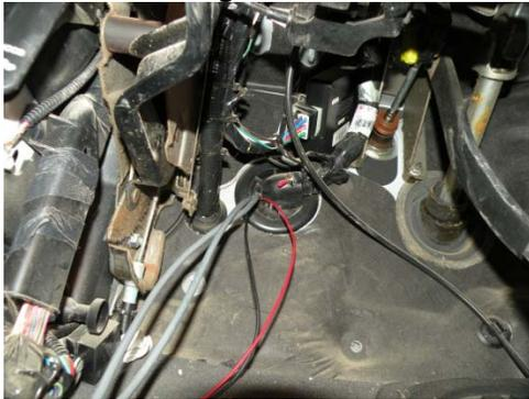
\*\*\* Be Sure To Insulate Wires Where They Enter Firewall, Failure To Do So May Cause SEVERE Damage To Controller, or To The Vehicles Computer System. \*\*\*
