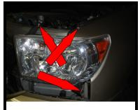
3.) Remove three bolts with a 10mm socket. Remove headlight housing. Carefully disconnect all harnesses from stock housing. Remove the two amber bulbs from stock housing and install them into new housing.
