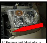
1.) Remove both black plastic rivets by prying up center portion with a flat head screwdriver.
